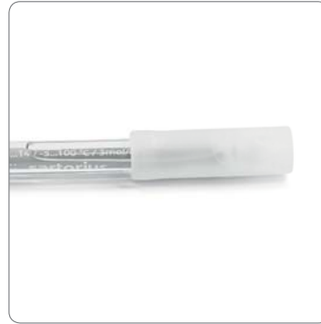
Removable Flushable Air Cap – eliminates clogs
